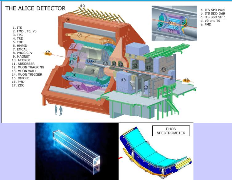
**ALICE** (A Large Ion Collider Experiment) is a heavy ion experiment on LHC at CERN. Its main goal is to study strongly interacting matter at extreme energy densities where the formation of a new state of matter, the quark-gluon plasma, is expected. RRC “**Kurchatov Institute**” manages the development and construction of Photon Spectrometer (**PHOS**) at ALICE.
